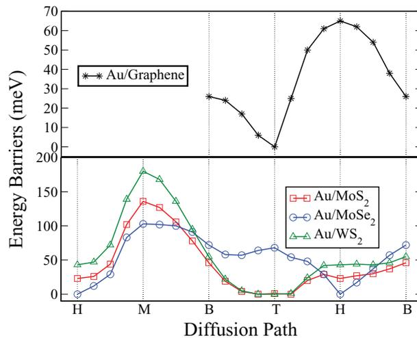
FIG. 3. Diffusion paths of Au on Graphene, MoS<sub>2</sub>, MoSe<sub>2</sub>, and WS<sub>2</sub>. (see Fig. 1 for sites.)
