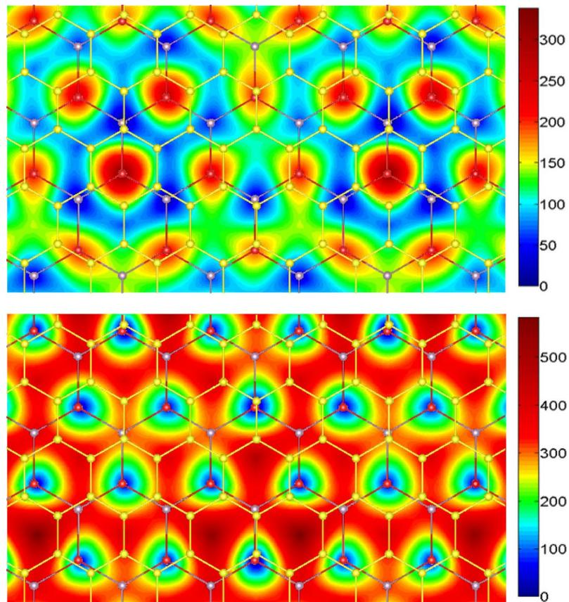
FIG. 4. Contour plots of the energy barriers (in meV units) seen by Ag (upper panel) and Au (lower panel) atoms intercalated in MoS<sub>2</sub>/Graphene heterostructure.
