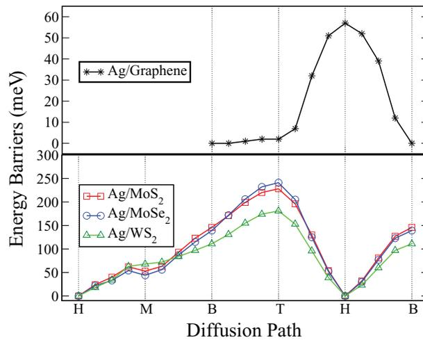
FIG. 2. Diffusion paths of Ag on Graphene, MoS<sub>2</sub>, MoSe<sub>2</sub>, and WS<sub>2</sub>. (see Fig. 1 for sites.)
